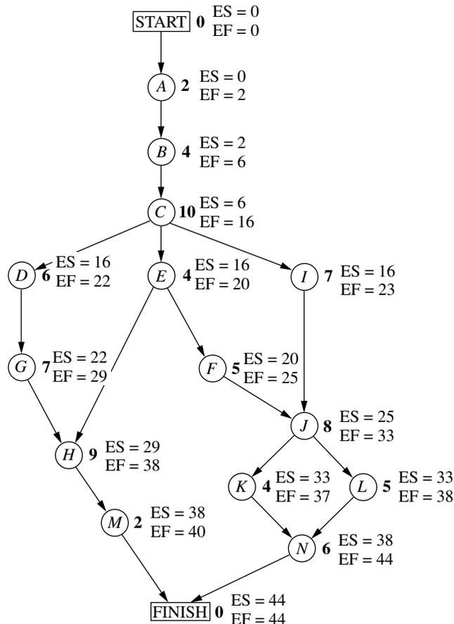
Note that Fig. 10.5 also includes ES and EF values for the START and FINISH nodes. The reason is that these nodes are conventionally treated as *dummy activities* that require no time. For the START node,  $ES=0=EF$  automatically. For the FINISH node, the earliest start time rule is used to calculate ES in the usual way, as illustrated below.
