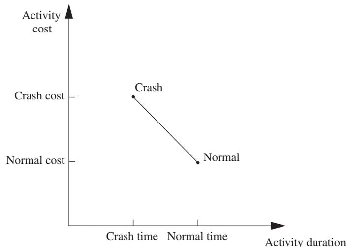
these two points. (For example, this assumption says that *half* of a full crash will give a point on this line segment that is midway between the normal and crash points.) This simplifying approximation reduces the necessary data gathering to estimating the time and cost for just two situations: *normal conditions* (to obtain the normal point) and a *full crash* (to obtain the crash point).
