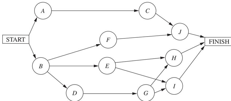
Using the PERT three-estimate approach, the usual three estimates of the duration of each activity have been obtained as given below.
